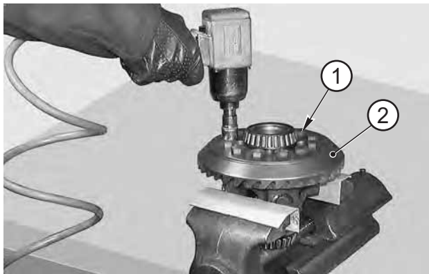
FIGURE 1: Remove the capscrews (1) from the crown (2).
