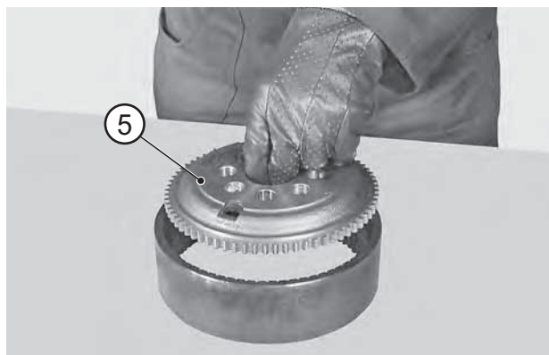
FIGURE 10: Remove the crown flange (5).
