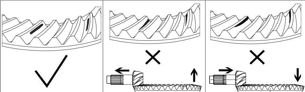
To make the bevel gear pair contact visible, apply a thin layer of bright paint on some teeth of the ring gear. Turn the pinion in both directions until the tooth contact pattern becomes visible. If the bevel gear adjustment is correct, the contact between the surfaces of the teeth will be optimal.
